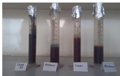
Figure 7: representation of modified media with crude oil, petrol, diesel and kerosene with culture 7
